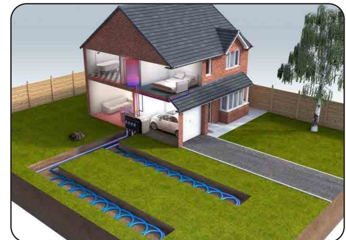
Figure 65: Example of a ground source heating system
